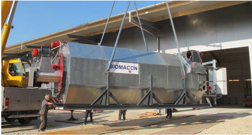
Abb. 02: Pyrolyseanlage Firma BIOMACON [Foto: Biomacon]
